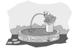
Water arcs high into the air from the mouth of a large, green stone frog and splashes cheerily into a surrounding pool. No matter how much water the frog spews out, the pool never overflows. Why not? Because a pump at the bottom of the pool pushes the water back up through a pipe to
