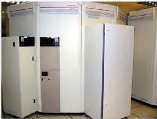
Above: A StorageTek PowderHorn Tape Library. Each library has a capacity of more than 5000 tapes and can mount 450 tapes an hour. Each has a capacity of up to 2 petabytes. Sandia currently has six PowderHorn libraries in production.
