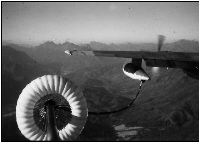
An HH-3E pilot's view from his helicopter "plugged into" a n HC-130P "tanker"
