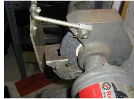
Picture 7 Bench Grinder with inadequate guarding
