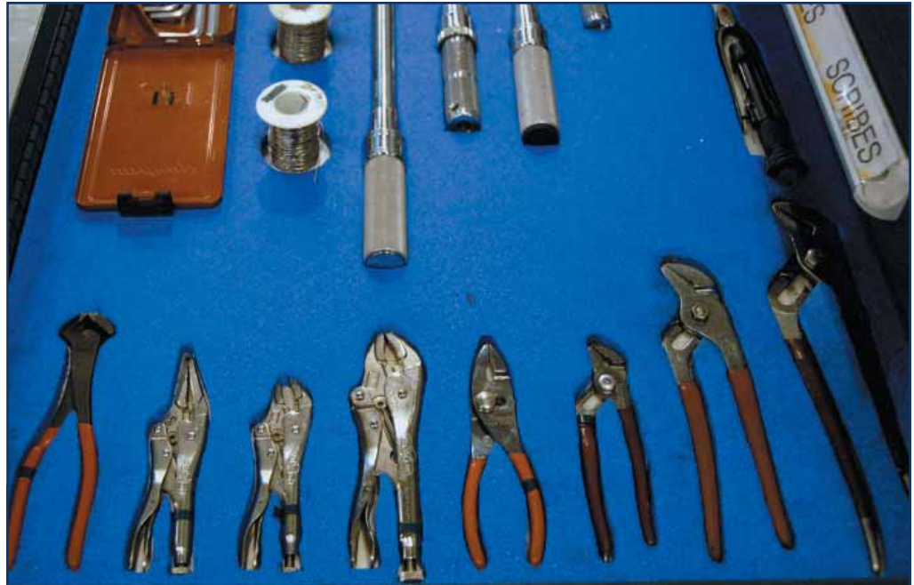
KODIAK, Alaska—At aviation maintenance facilities throughout the Coast Guard, such as Air Station Kodiak's MH-60 maintenance department, disciplined processes are the norm. For example, tools are kept in form-fitting trays, organized for accountability and easy access by technicians. Coast Guard Photo by Petty Officer 3rd Class Richard Brahm
