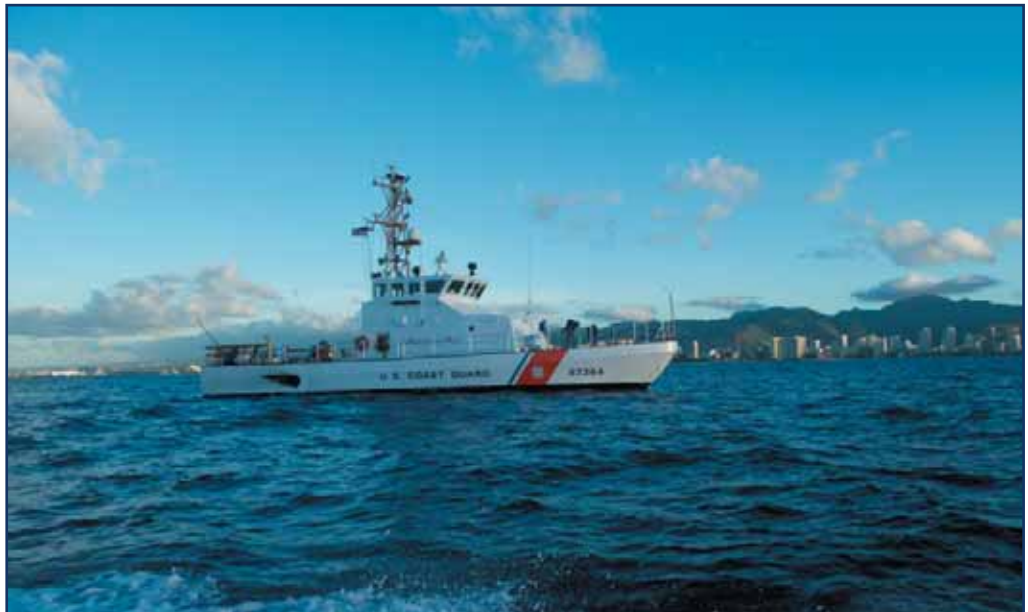
USCGC Ahi patrols the coast off of Waikiki Beach, Hawaii. The 87-foot Marine Protector-class cutters are designed to operate in heavy seas (up to sea state 5), and equipped to handle a variety of Coast Guard missions. U.S. Coast Guard photo by Petty Officer First Class C.C. Clayton
