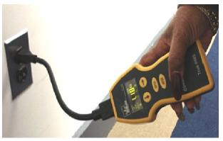
Figure 1: Impedance Tester
