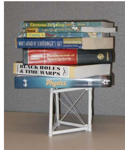
Model truss structure of flimsy paper and kite string is strong enough to support all these heavy books!
