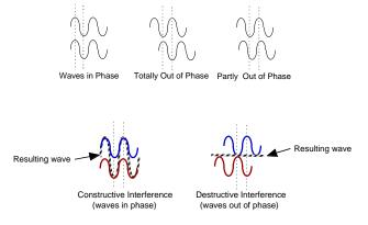
As wave fronts interact, constructive and destructive interference creates characteristic patterns. Understanding wave behavior through the observation and measurement of interference patterns is called interferometry.
