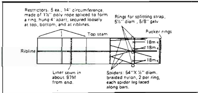
Figure A.- -Schematic diagram of the 90-105 polyethylene Nor'eastern bottom trawl, roller gear and accessory gear used during the 1990 Gulf of Alaska bottom trawl survey from 4 June to 9 September 1990.
