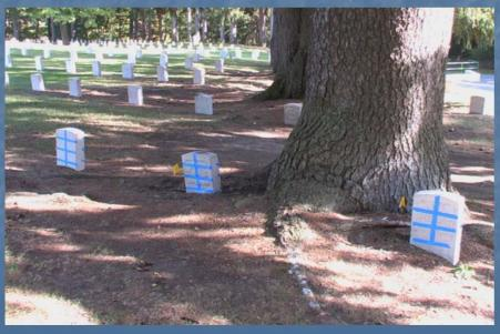
Selected headstones are intentionally located in both shaded and sunny locations, to test for the environmental variable of light.
