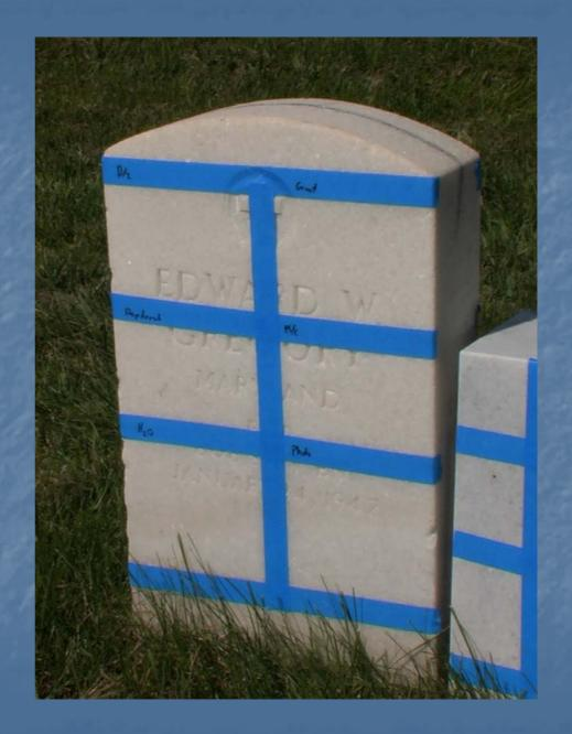
The five cleaners being tested reflect a variety of active ingredients and potential sources of marble damage. The products being tested are.
