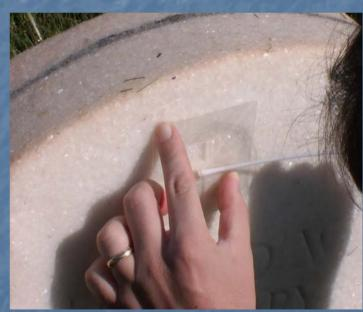
Taping a headstone and a lab sample (right) with a low-adhesive tape creates six test plots on the front and back sides of each.
