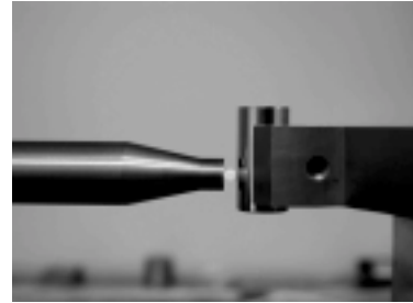
Ferrule diameter measurement with laser micrometer.
