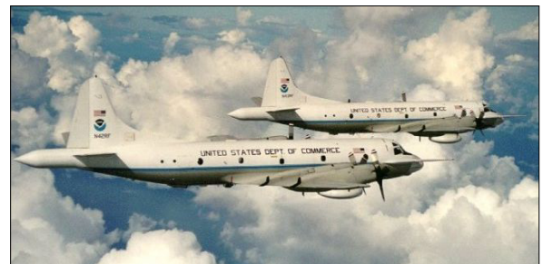
NOAA's P-3 Orion aircraft are a key component of HRD's hurricane field program. The specially-instrumented aircraft serve as airborne observing platforms, enabling researchers to gather data from the inner core and surrounding environment of tropical cyclones.
