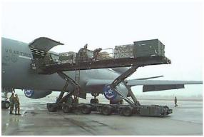
The Air Force uses the 60K Tunner cargo loader to load and unload cargo from military and commercial transport aircraft. The loader, managed by the Warner Robins Air Logistics Center (WRALC), can handle up to 60,000 pounds of cargo. The Air Force procured 318 Tunner cargo loaders between FYs 1997 and 2005.
