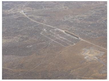
roadside barrier, tracer measurements were made on two separate grids so that results could be compared. These two grids were identical to each other with the exception that one grid had the barrier and one did not. They had a large crosswind separation to eliminate any possible interference.
