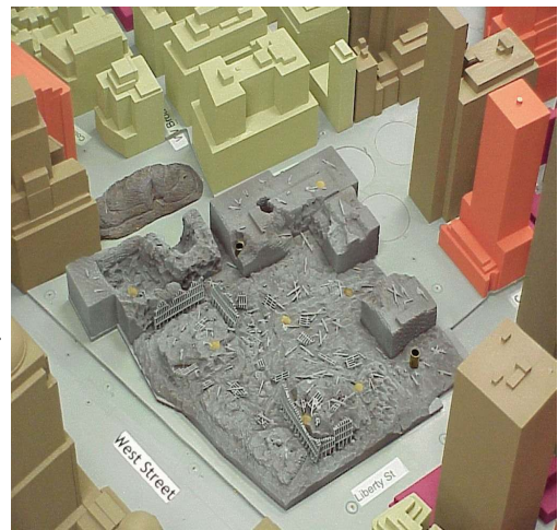
Figure 1: Model constructed for wind tunnel tests.
