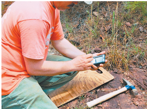
USGS hydrologist at a quartzite-schist outcrop entering structural data into a handheld computer. The USGS, working with the State University of West Georgia, has developed a system for digital collection of structural data into a handheld computer and a global positioning system receiver. Photo by Ethan W. Williams
