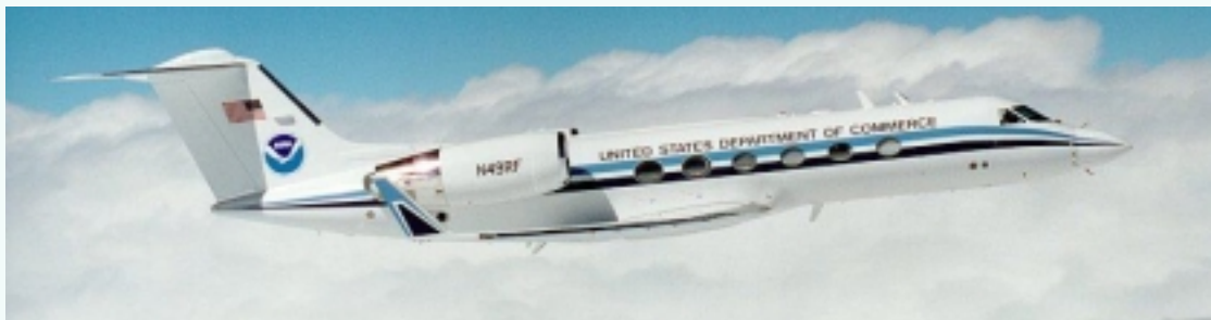
NOAA's Gulfstream-IV SP jet is a state-of-the-art high altitude research platform. It was acquired in 1996 to improve NOAA's tropical cyclone forecast capability by being able to deploy dropsondes from high altitudes over large areas of open sea, where few observations are available.
