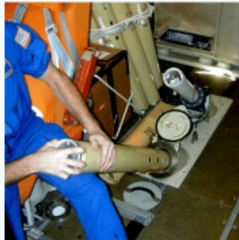
An airborne expendable bathythermograph (AXBT) is launched from one of NOAA's WP-3D reconnaissance aircraft.
