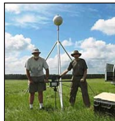
NOAA scientists setting a ground anchor for an Extreme Turbulence Probe deployed in advance of Hurricane Ivan. Photo: NOAA
