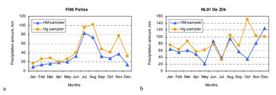
*Fig. 3.5.* Precipitation amounts collected by sampler for heavy metals (blue) and by sampler for mercury (orange): a) – site FI96; b) – site NL91
