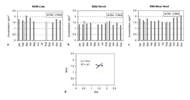
Fig. 7.2.1. Comparison of measured and calculated by CMAQ concentrations of gaseous elemental mercury (GEM) at EMEP sites
