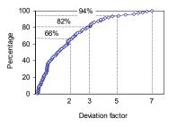
Fig. 7.3.5. Cumulative distribution of deviation factors for the totality of wet deposition results obtained by EMAP (9 stations, 12 months)
