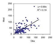
Fig. 7.4.3. Monthly mean forecasted precipitation amounts used by MSCE-HM against observed precipitation amounts measured at the monitoring stations, mm
