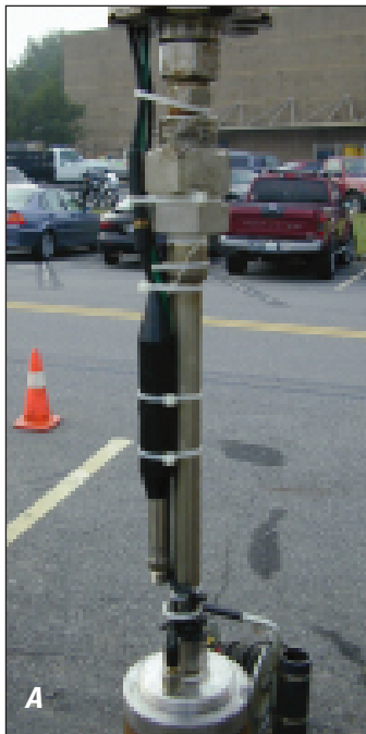
Figure 13. AFP6 straddle packer: (A) middle transducer situated between shroud and lower packer, (B) tubing and cable connections between middle packer and shroud, and (C) down-hole tubing affixed to drill rod during packer deployment.
