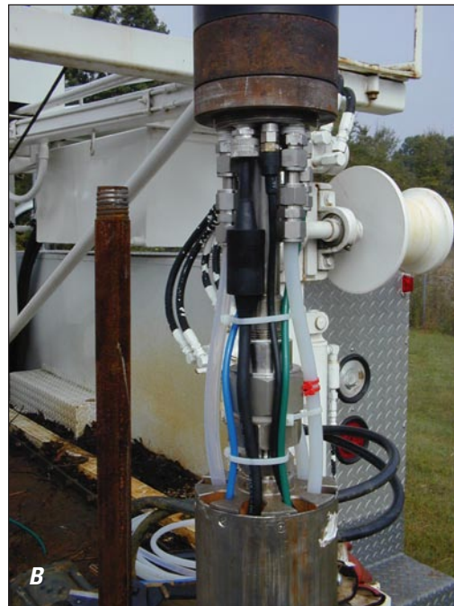
Figure 13. AFP6 straddle packer: (A) middle transducer situated between shroud and lower packer, (B) tubing and cable connections between middle packer and shroud, and (C) down-hole tubing affixed to drill rod during packer deployment.
