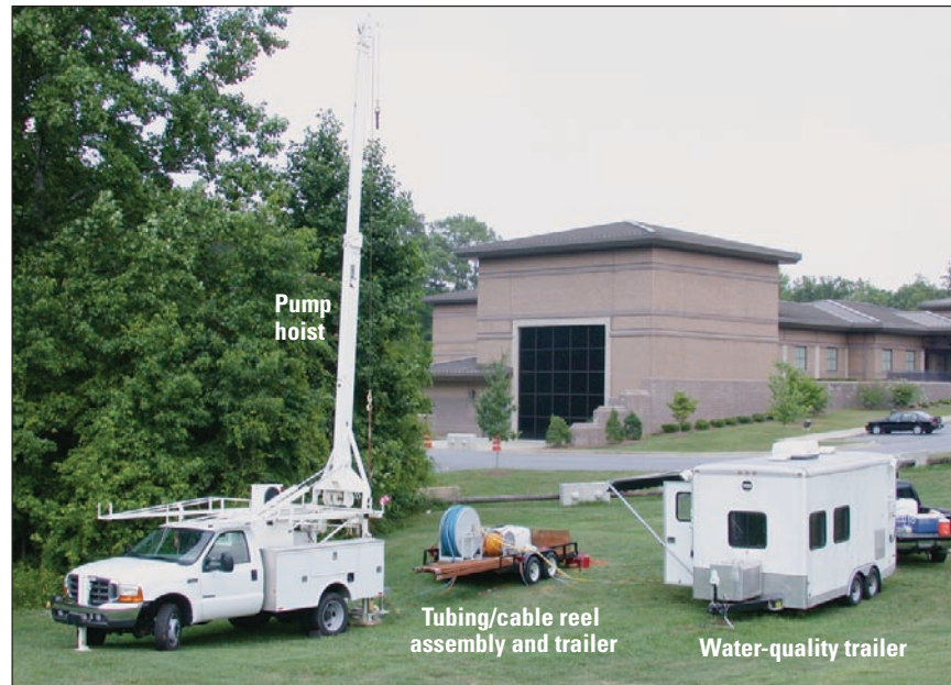
Figure 5. Components of AFP6 straddle-packer system, U.S. Air Force Plant 6, Marietta, Georgia.
