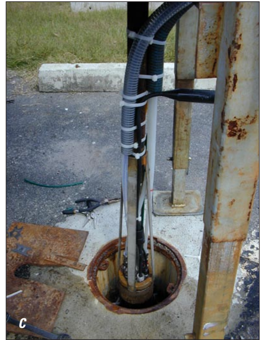
Figure 13. AFP6 straddle packer: (A) middle transducer situated between shroud and lower packer, (B) tubing and cable connections between middle packer and shroud, and (C) down-hole tubing affixed to drill rod during packer deployment.
