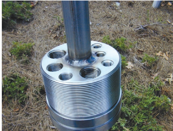
Figure 12. Head of upper packer showing custom drilled and tapped holes to accommodate two 1/2-inch pneumatic lines, one 5/8-inch discharge line, three 1/4-inch pneumatic lines, a single transducer cable, and a power-supply cable for the electrical submersible pump, AFP6 straddle packer.
