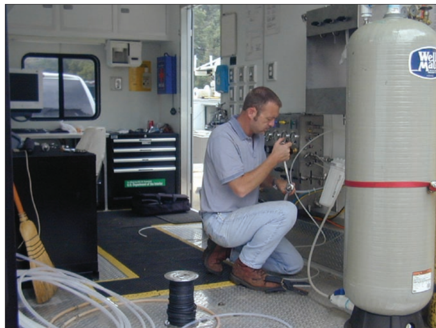
Figure 6. Interior of water-quality trailer. The tank to the right contains deionized water used for borehole injections.
