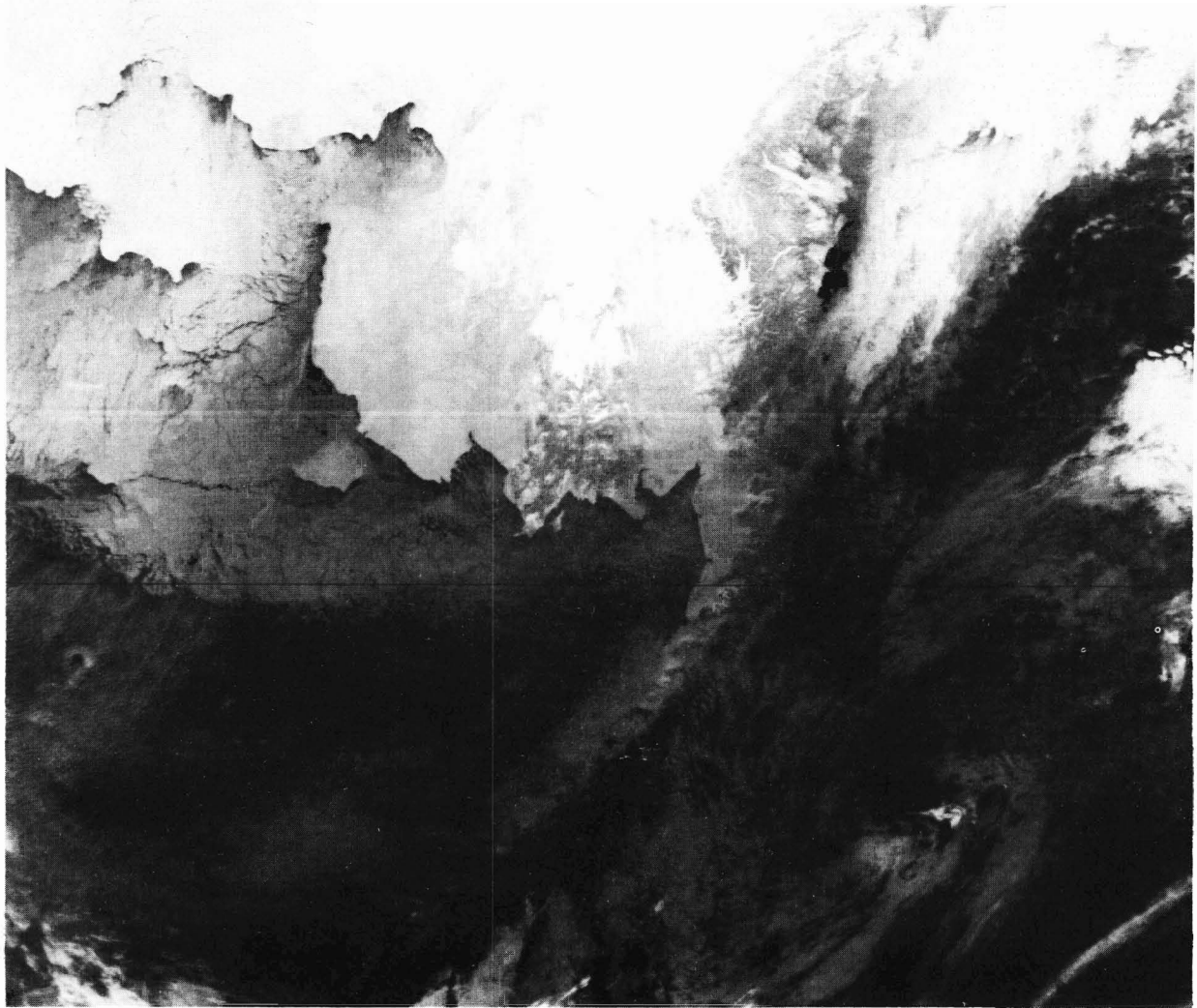
Figure 7.—Ice cover in the eastern Bering Sea, 18 February 1983, NOAA-7 AVHRR channel 4. Ice, clouds, and snow-covered land all appear whiter (colder) than open water. Pack ice extends from the Bering Strait, in the top left corner, past St. Matthew and Nunivak Islands, but does not reach the Alaska Peninsula to the southeast. Photograph courtesy of G. L. Hufford, NOAA/NESDIS, Satellite Field Services Station, Anchorage, Alaska.
