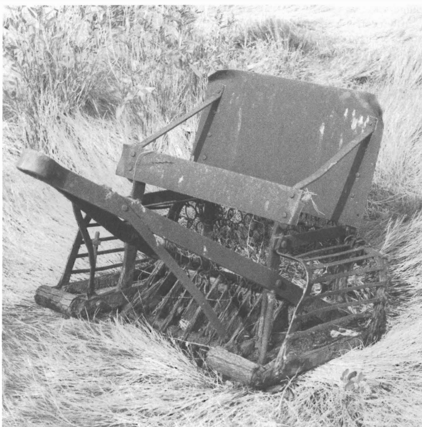
Figure 28.—A rocking chair dredge for hard clams, 1988. Photograph by the author.
