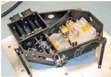
Brassboard internal metrology beam launcher: successfully passed vibration and thermal tests; passed metrology stability and cyclic error requirements at the 3 \mu\text{m} level. Will be integrated into the ABC in 2009.
