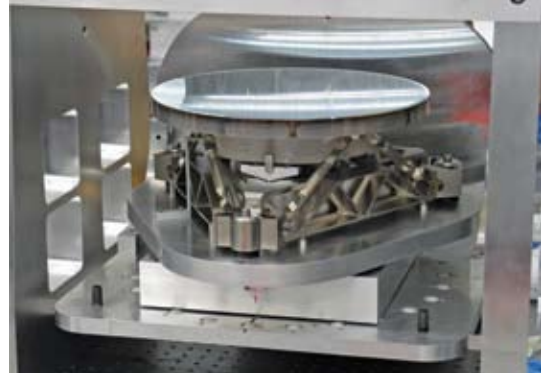
Prototype primary mirror assembly (M1): figured and mounted a 300 mm lightweight mirror with 5.7 nm RMS wavefront error. Successfully passed both vibration and thermal tests.
