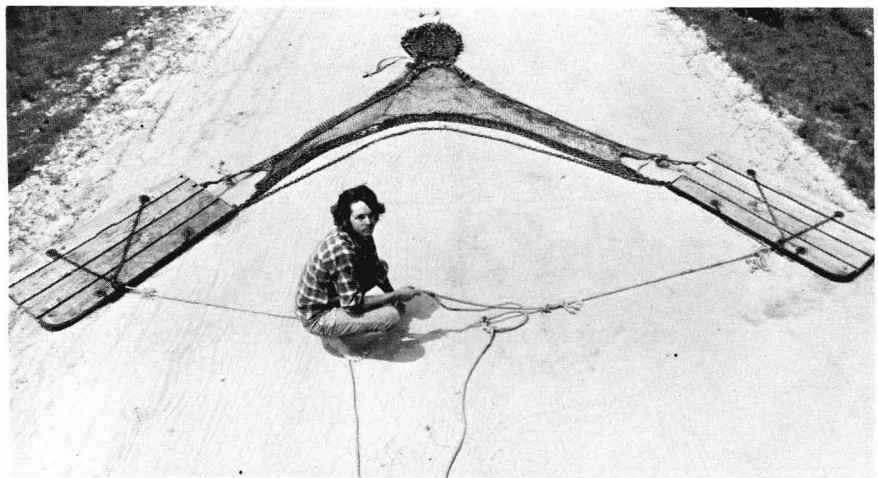
Figure 7.—The clam trawl, with boards attached.
