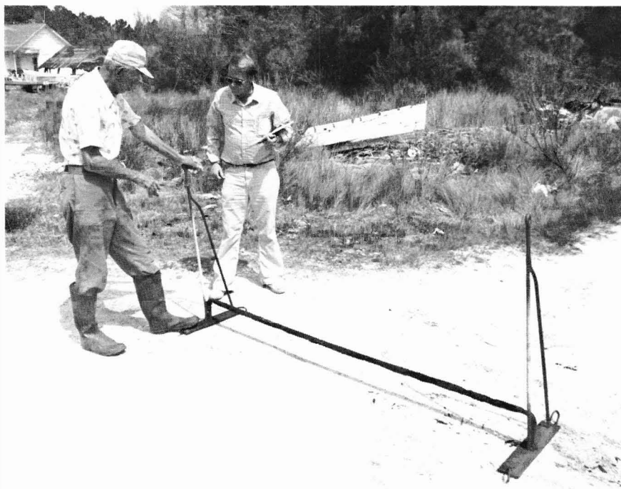
Figure 3.—The basic bedstead frame, to which a trawl net was attached.
