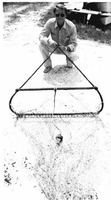
Figure 5.—The oyster drag with bunt attached.
