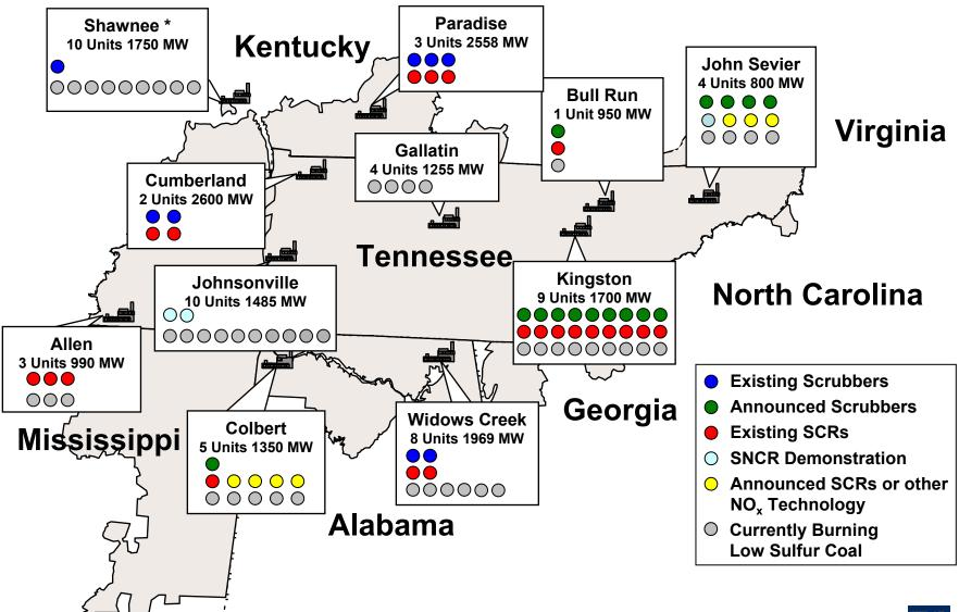
\* Shawnee Unit 10 is an Atmospheric Fluidized Bed Combustion (AFBC) boiler which lowers SO<sub>2</sub> and NOx emissions without the use of external controls. NOTE: In addition to 21 selective catalytic reduction systems, TVA has installed low NOx burners or over-fire air on 40 of the 59 coal-fired units. The other units have installed boiler optimization systems and Shawnee Unit 10 is a boiler with low NOx technology.
