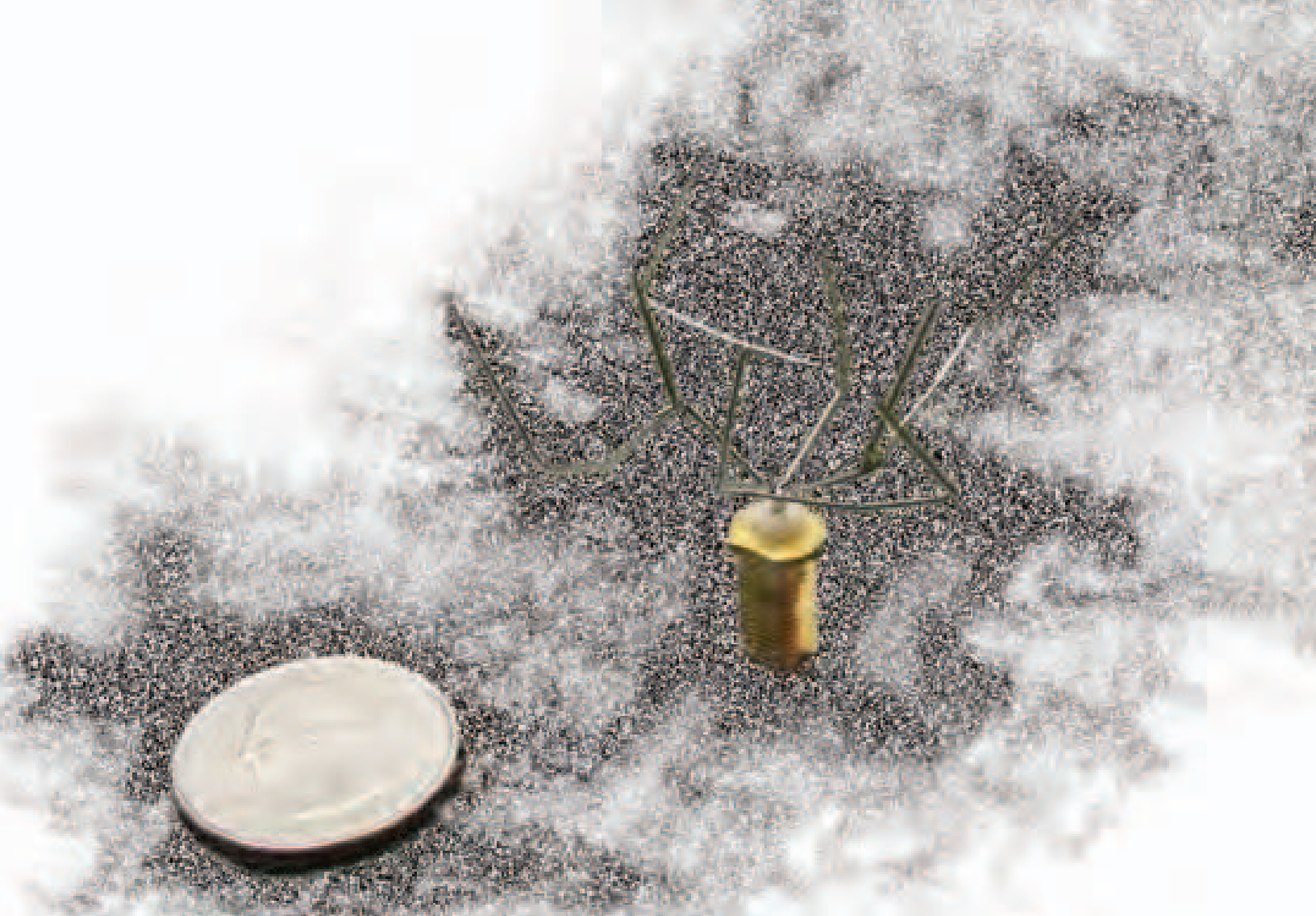
An antenna designed by a computer might become the first piece of evolvable hardware in space in 2004.
