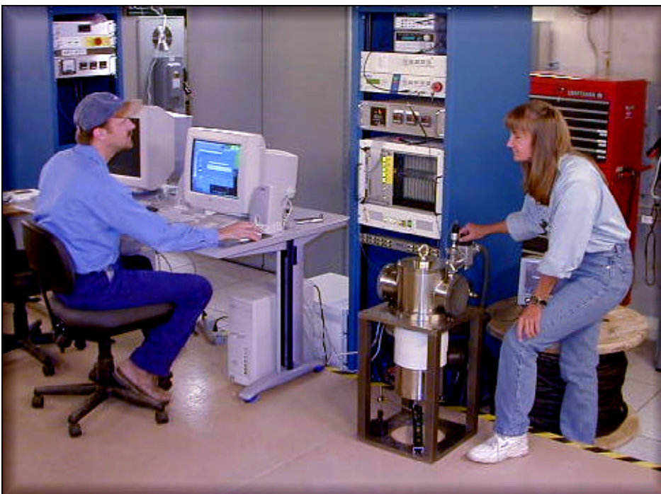
Argonne technicians Ray Ziegler and Lynette Jirik in the Argonne chopper lab carrying out acceptance testing for the E_0 chopper prototype.
