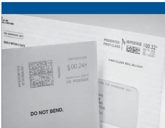
The Information Based Indicia (IBI) is a digital imprint that is valid postage. IBI contains the date, class of mail, postage amount, originating ZIP Code, and a unique device identification number.
