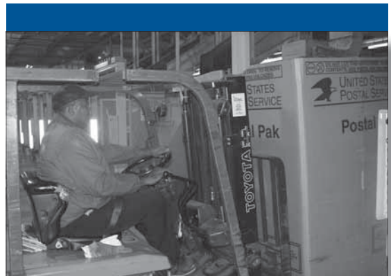
The Postal Service uses various types of vehicles within plants to move mail from one location to another during processing. Pictured here is a Powered Industrial Vehicle.
