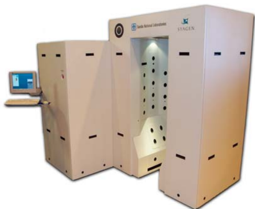
Prototype Portal using Mass Spectrometry Detection
