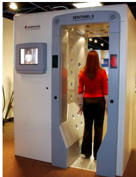
Commercialized Version of Explosives Detection Personnel Portal with IMS Detection
