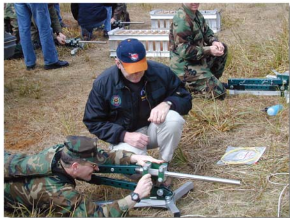
Bomb squad personnel learn to use the Percussion-actuated Nonelectric (PAN®) Disrupter
