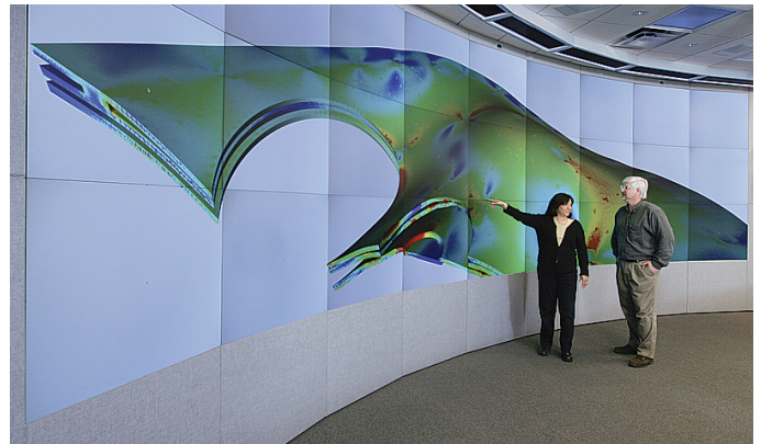
Small details in complex models and simulations become apparent when viewed on the IDC's 35 million pixel main display.
