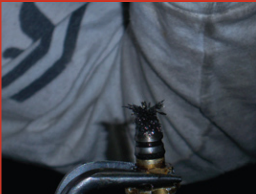
AMAD chip detector (not supposed to have all the metal filings on it).
