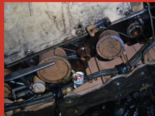
AMAD oil transducer cap blown off of the bottom of the AMAD.
