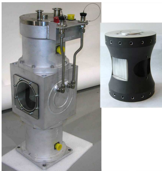
Fig. 5.12. Left: photograph of ARCS Fermi chopper, showing housing, windows, and water cooling. Right: photograph of the slit package, with aluminum slits seen end-on.
