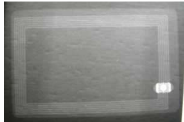
X-ray confirms the hidden RFID chip and antenna
