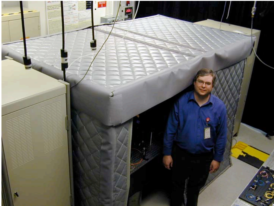
Figure 3: View of the Adaptive Nuller after the installation of its acoustic enclosure (January 29, 2009). The enclosure was installed for this milestone and reduced the measured ambient acoustic noise by more than 15 dB. The testbed PI, Robert Peters, is shown in the foreground. The enclosure was manufactured by DB Engineering.
