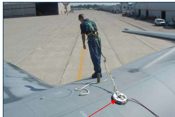
Vacuum pads are compressed against the aircraft skin by atmospheric pressure and held in place due to the negative pressure beneath the pads.
