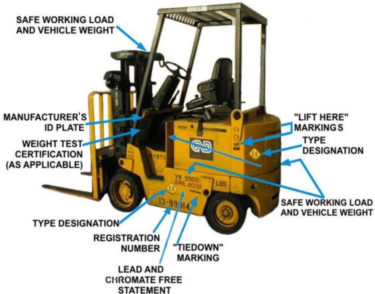
FIGURE 5-5. Shorebase Electric Forklift Truck Markings (Example)
