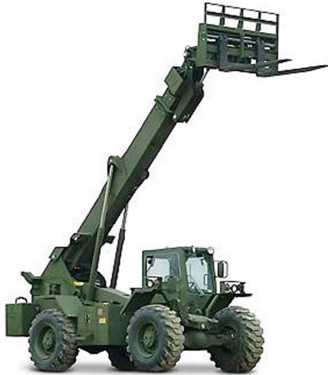
FIGURE 3-9. Rough Terrain Forklift Truck (Variable Reach Boom-Type)
