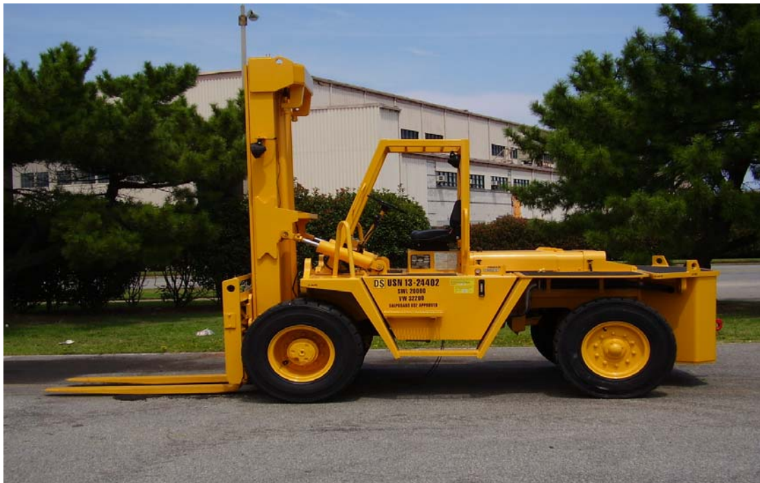
FIGURE 3-3. Standard Profile Shipboard Diesel Forklift Truck
