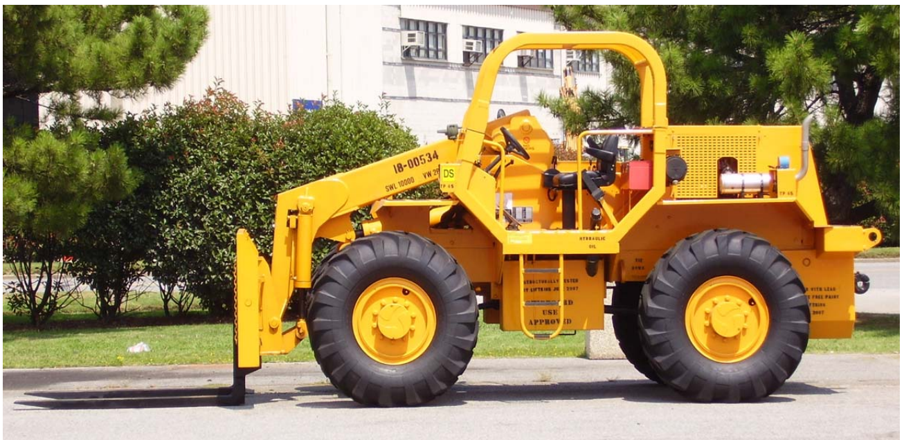
FIGURE 3-7. Rough Terrain Forklift Truck (Vertical Mast)
