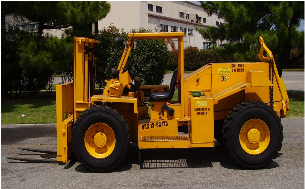
FIGURE 3-7. Rough Terrain Forklift Truck (Vertical Mast)
