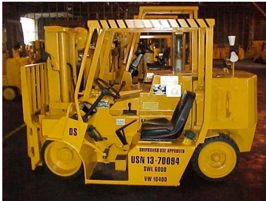
FIGURE 3-2. Low Profile Shipboard Diesel Forklift Truck
