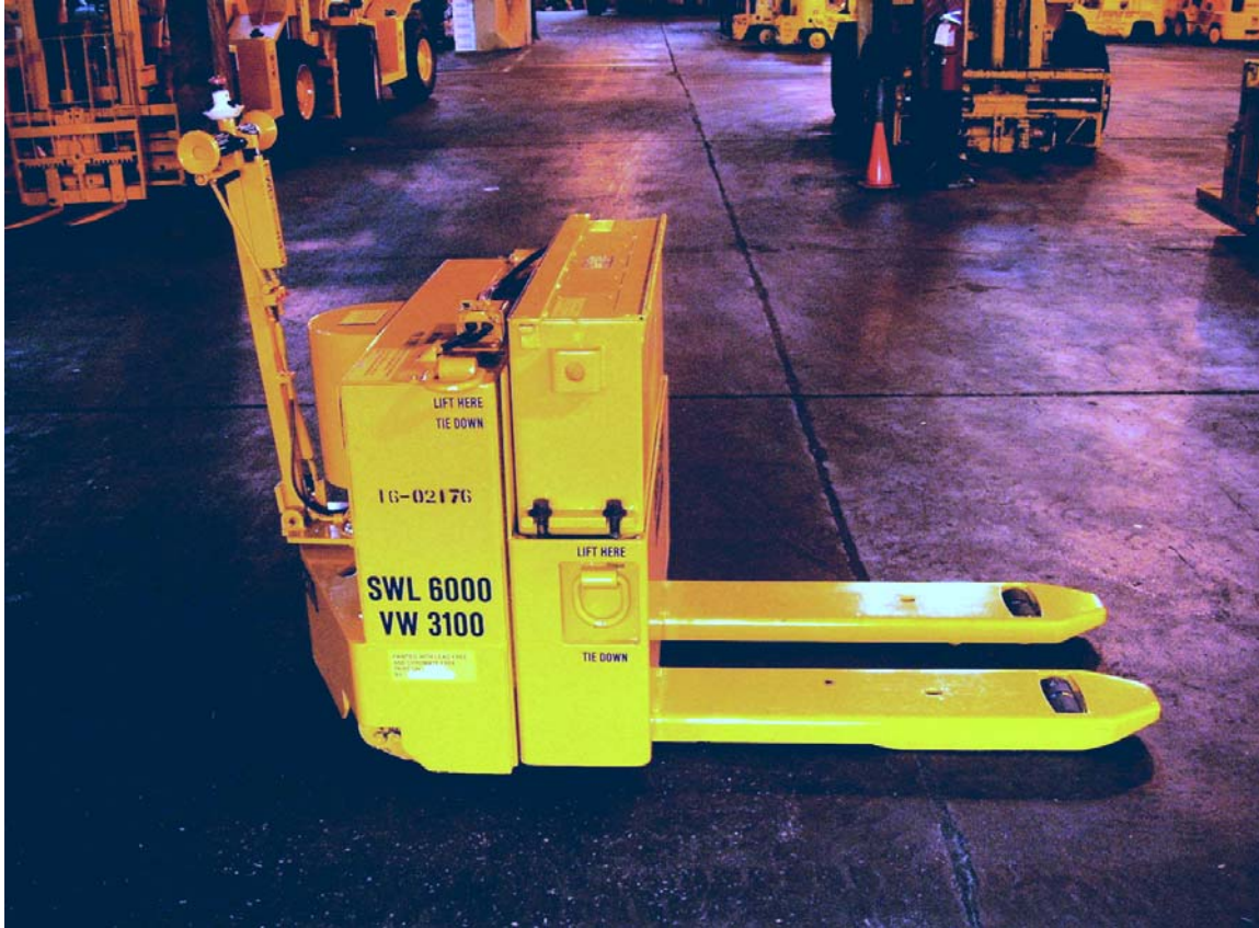
FIGURE 3-15. Electric-Powered Walkie-Type Pallet Truck
