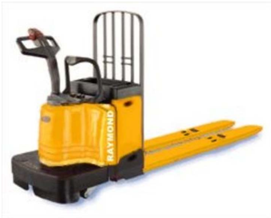
FIGURE 3-14. Electric-Powered Rider-Type Pallet Truck
