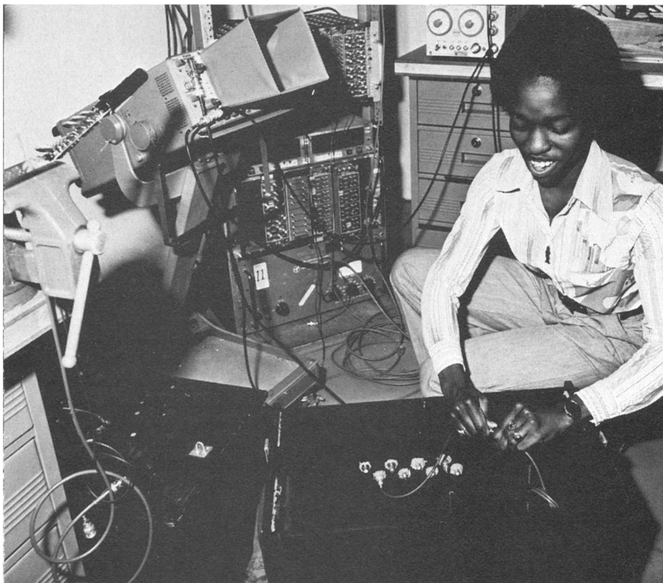
Fig. 1. Carolyn Alexander from Virginia State College working on development of a counter hodoscope for the Fermilab single-arm spectrometer.
