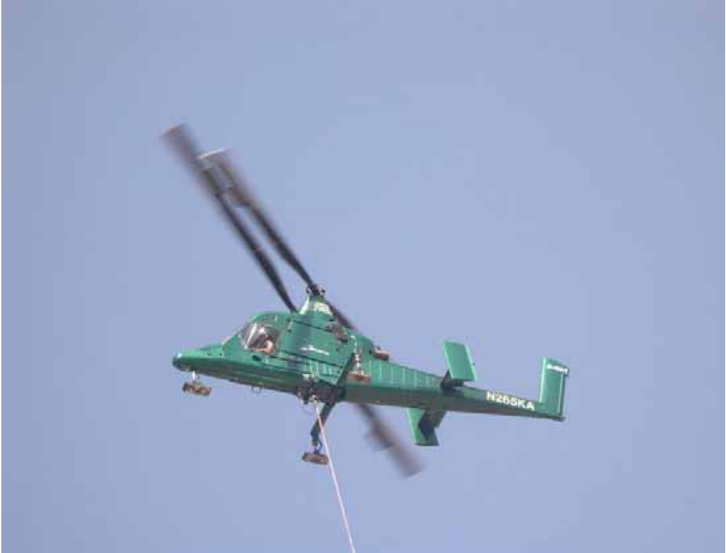
Figure 9 - KMAX Helicopter used to transport equipment to worksite.
