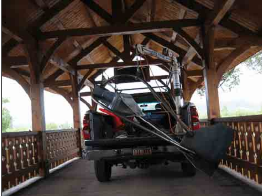
PHOTO 4.6. BIO-WEST'S 6-INCH HELLEY-SMITH-TYPE CABLE SUSPENDED BEDLOAD SAMPLER.
