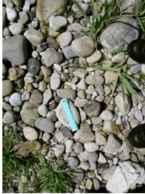
Photo of patch at NC site near PC#1 (blue 152mm ruler for scale): 30% cobble, 35% large gravel, 35% medium gravel
