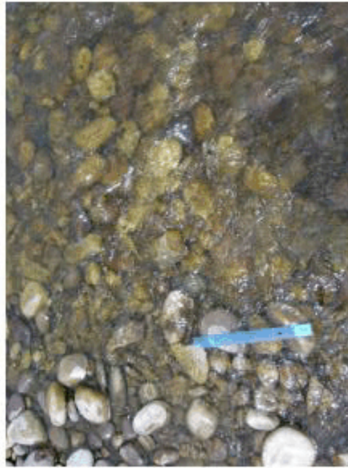
Photo of patch at CA site near PC#2 (blue 300 mm ruler for scale): 40% cobble, 35% large gravel, 25% medium gravel
