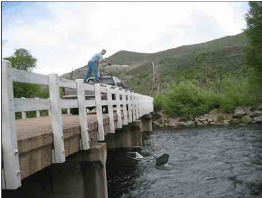
PHOTO 4.7. BIO-WEST'S 6-INCH HELLEY-SMITH-TYPE BEDLOAD SAMPLER IS LOWERED FROM THE WHITE BRIDGE (WB) MONITORING BRIDGE USING AN AUTOCRANE.
