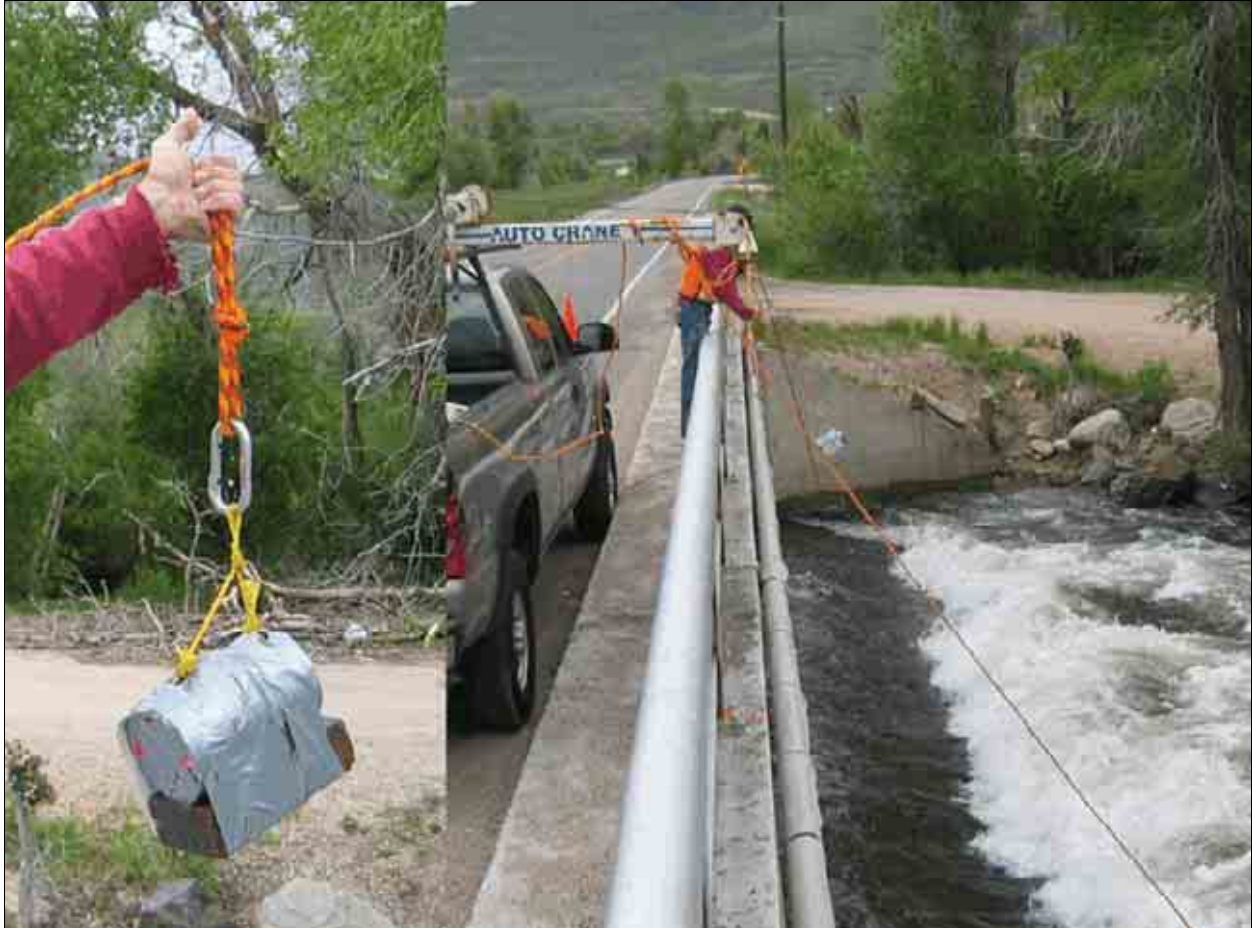
PHOTO 4.5. PHOTOGRAPH OF THE DEVICE USED TO OBTAIN SUSPENDED SEDIMENT (TSS) SAMPLES FROM BRIDGES.
