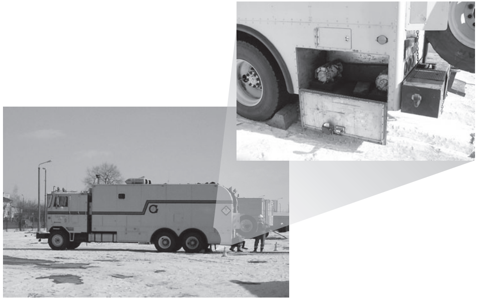
Figure 4: Unsecured Transportation Vehicle Containing Radiological Sources
