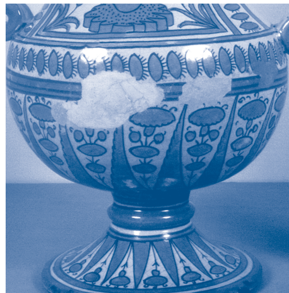
Figure 1. Ceramic object with glaze loss
