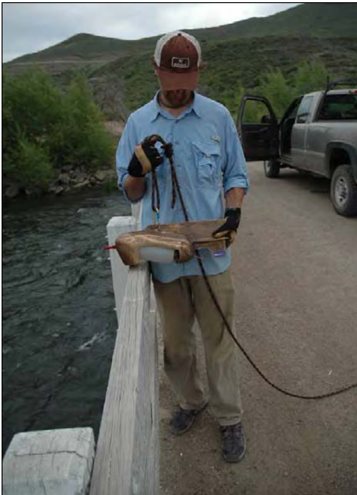
Photo 4.1. Depth-Integrated Hand Line Model US DH-76 and sampler holder.
