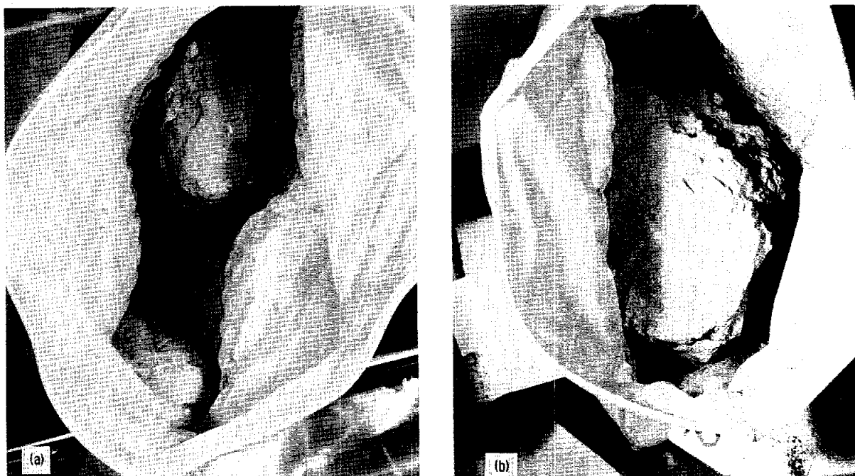
FIGURE 7-21.—Padded bag samples during cursory inspection. (Only the top was opened; the rocks were left untouched.) (a) Sample 67215 (bag 1) appears to be a moderately tough, polymictic breccia, and considerable dust has accumulated on the inner walls of the bag and on the bottom. (b) Sample 67235 (bag 2) is a hard breccia, probably of the recrystallized dark matrix type. Some soil was present on the bag walls, although considerably less than in padded bag 1. Both rocks are dust covered, which prevents a more detailed description at present. The rocks await special processing.
