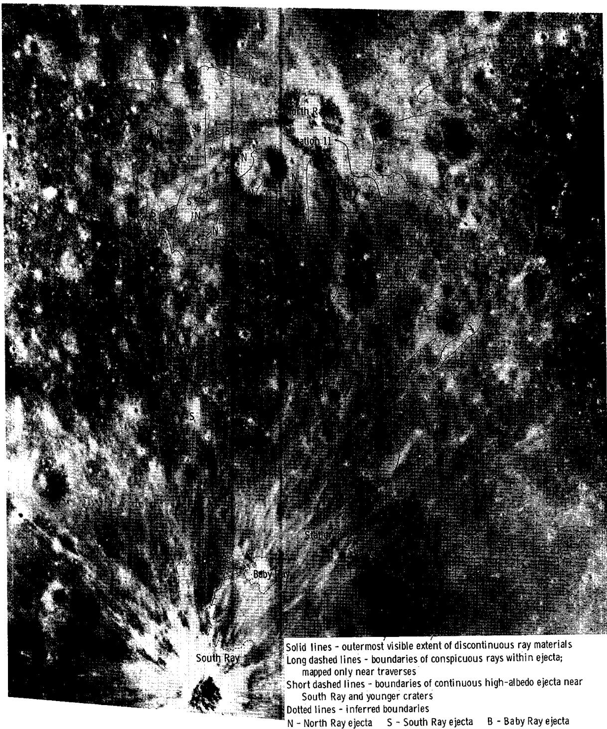
FIGURE 6-5.—Map of ejecta distribution in the Descartes landing site area. Derived from second-generation film positives of Apollo 14 orbital photographs AS14-69-9520 and 9522 (500 mm), using stereographic analytic plotter.
