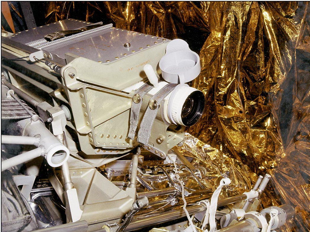
Westinghouse Color Camera in MESA mount, with the added lens cap, before Apollo 13 LM Closeout
