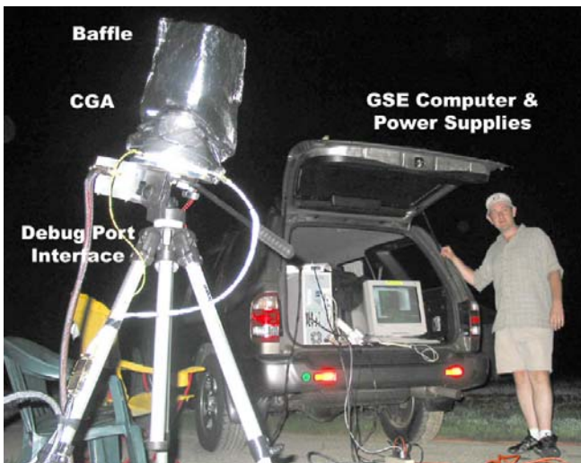
Figure 6 – Typical CGA-only night sky test setup at MIT Wallace Observatory in Westford, MA. The CGA is bagged for protection from condensation and insects.
