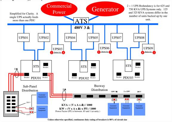
This is a typical n+1 power distribution model. Power enters the building either from the commercial power grid or a generator through an automated transfer switch (ATS). The ATS is responsible for determining if the commercial power is stable. If not, the ATS will start the generator, determine that the power from the generator is stable, match the phase of the commercial power if it is available, introduce the power to the internal power distribution and shunt the commercial power feed.
