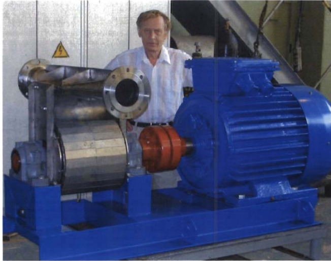
Fig. 3.7. Prototype permanent magnet mercury pump developed for the ESS.
