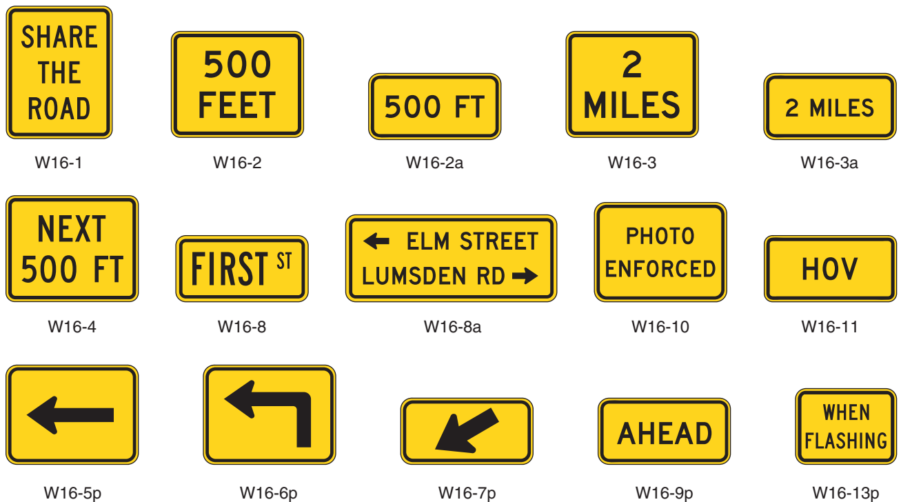
Figure 2C-11. Supplemental Warning Plaques
